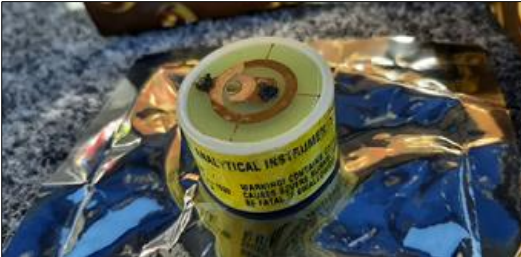
Figure 11: A faulty oxygen sensor from the system.
