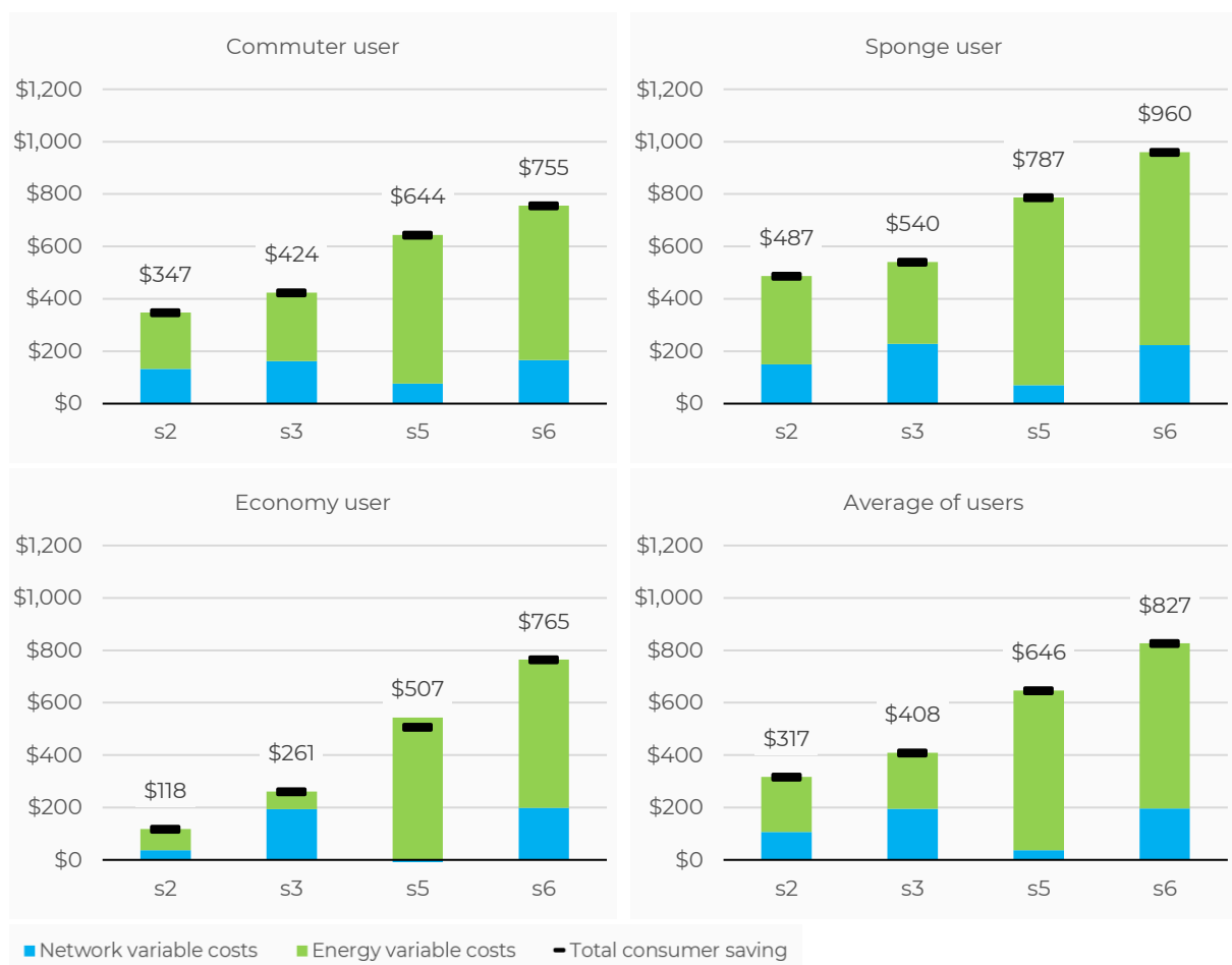
Figure 26 – Reduction in annualised electricity costs in moving from smart charging to V2G under each scenario, by customer type
