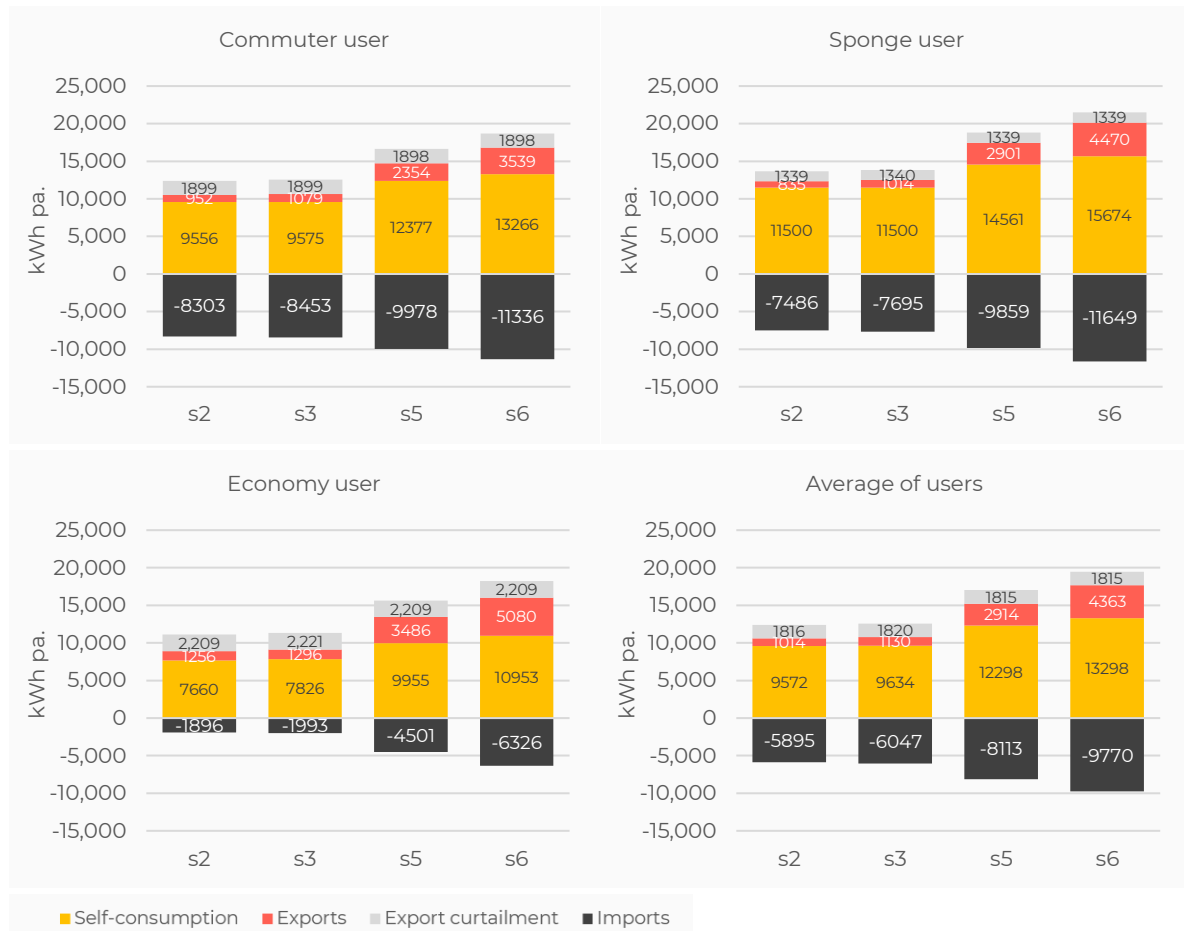
Figure 28 – Breakdown of total annualised customer electricity import and exports for V2G users under each scenario, by customer type (includes household loads and solar).
