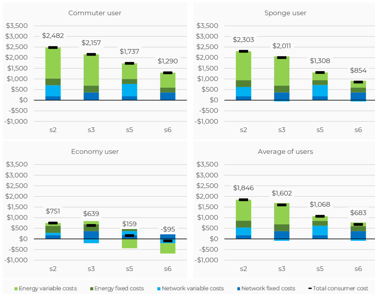
Figure 27 – Breakdown of total annualised customer electricity costs for V2G users under each scenario, by customer type (includes household loads and solar)
