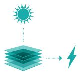
Tandem Solar Cells offer the promise of an efficiency boost, by stacking two solar cells, one on top of the other, to make the most of the available sunlight and deliver more power per unit area.
