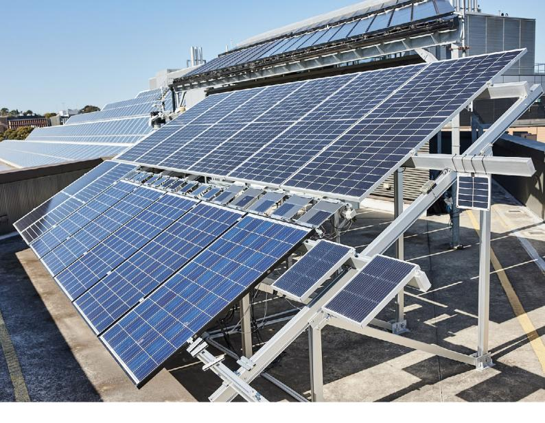
Solar cells under testing at UNSW.
