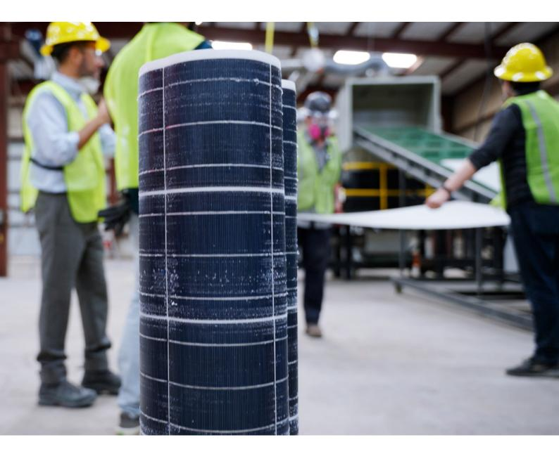
Laminate after the glass has been fully removed. Over 50% of the material value of a solar panel is in this fraction.
