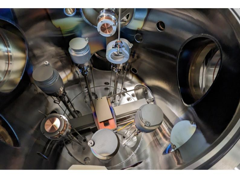
New sputtering system with chamber open, exposing the targets.
