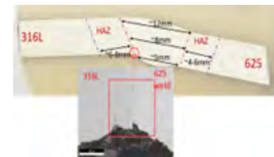
Inconel 625 & 316L weld exposed at 750°C/500 hr - QUT
