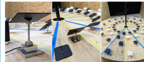
University of Adelaide indoor wind load testing - UOA
