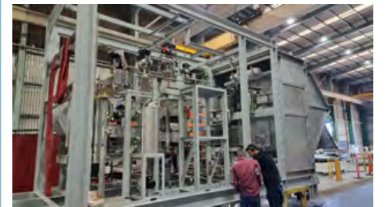
Sodium Test Loop Module under construction, Dec 2022 - CSIRO
