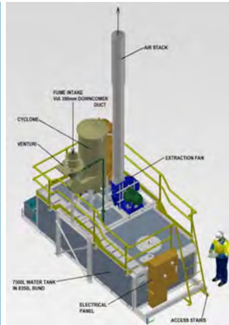
Final Engineering Design: Fume Scrubber System - CSIRO
