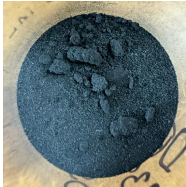
Figure 12 Clumps were formed in the processed G0114 DRI at 1050°C.
