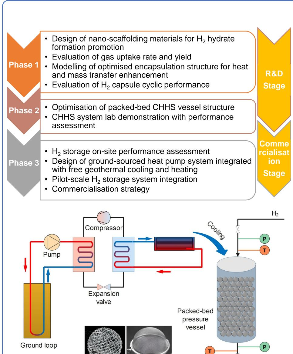
Schematic of the pilot-scale CHHS system
