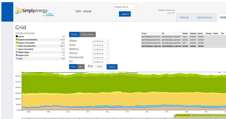
Figure 11: Snapshot from inGrid VPP platform providing view of demand and supply by type including DER.
