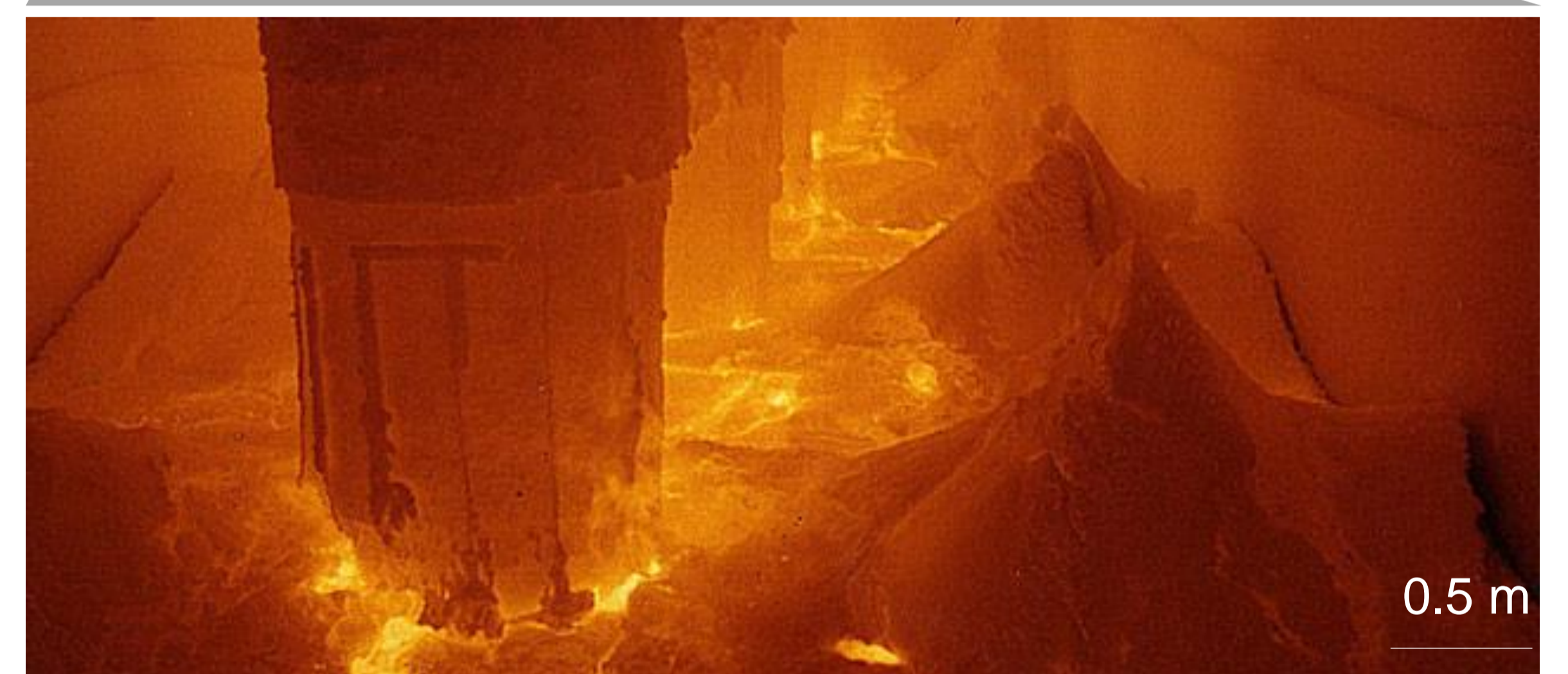
Melting bath in an operating ESF for iron sands ( https://teara.govt.nz/en/iron-and-steel )
