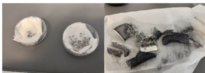
Figure PP5.5.4: Pictures of manually dismantled cells and hot-knife cells following submersion in organic solvents.
