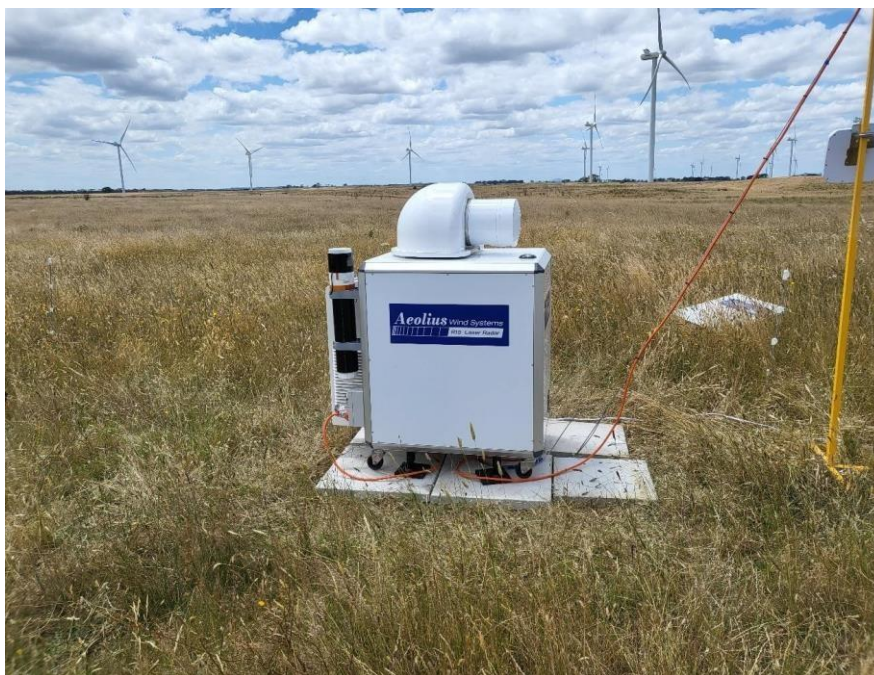
Figure 1 The Aeolius Wind Systems Long Range Doppler Lidar Forecaster (System No. 1) at Macarthur Wind Farm, December 2023. The turn-key lidar performs all required tasks to generate the forecast within the system itself thus avoiding potential security breaches with data products and removing reliance on third-party service providers.
