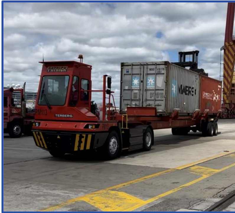
Figure 2: BEV- TT Commissioning operations at Patrick Terminals Fremantle
