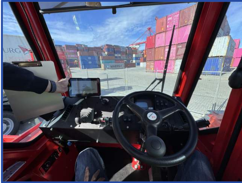
Figure 5: Prototyping driver interface screen as part of the Fleet Power Management System
