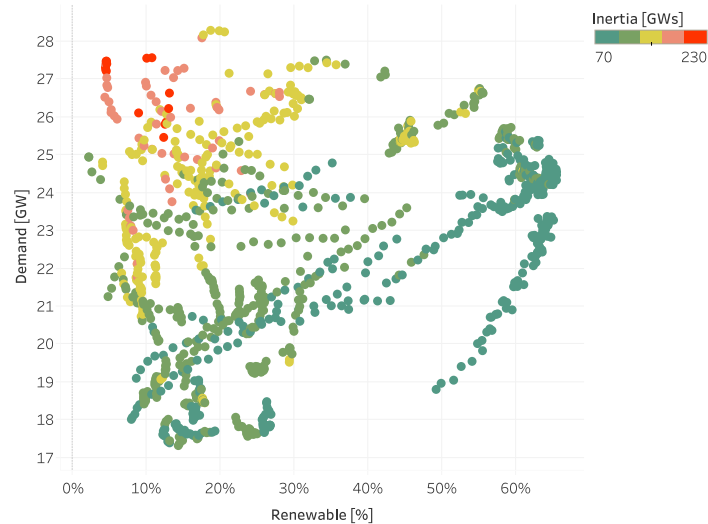
Figure 17 Inertia by renewable penetration and demand level
